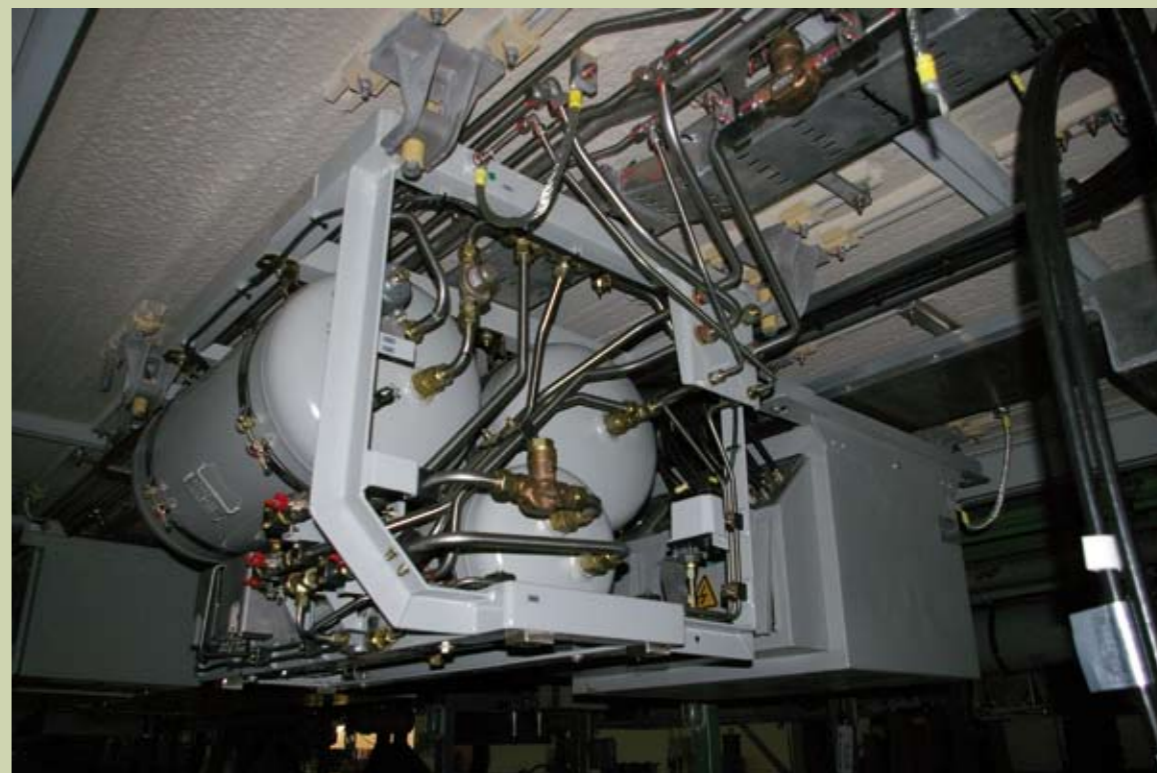
Traditional central sub-frame with reservoirs and piped components. EP2002 Cube replaces the visible lengths of piping with the boring in the cube.
