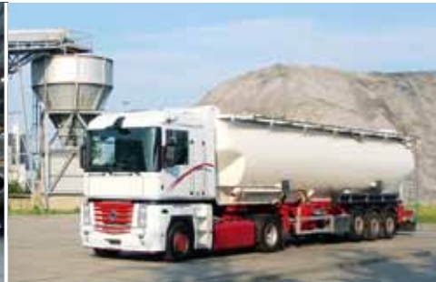
Container production at the Winsen plant. Silo articulated lorry with Feldbinder semi-trailer for bulk materials from the construction industry.
